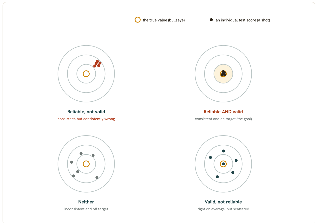
Fig 6.2 Reliability versus validity, the classic marksman analogy. Reliability is how tightly the shots cluster (consistency); validity is whether they land on the bull (accuracy). The two are independent: a test can be reliable but not valid (tight but off target, the dangerous case of a precise wrong answer), valid but not reliable (centred on average but scattered), neither, or both. The one dependency is that validity requires reliability, so a good test must be reliable first, then shown to be valid.
